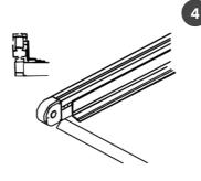
PVC profile pressed on the lateral side of the runner for retention of rainwater spray. Always in addition to the anti drop system.
