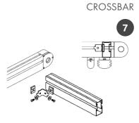
Aluminium profile and accessories to be fixed to self-supporting drive or, in addition, to support the protection cover.
