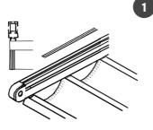
Welded PVC profile on the underside of the fabric. Only for fabrics in the suggested configuration.
