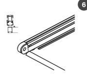
Weldable PVC profile on the upper part of the fabric for lateral rainwater prevention.
