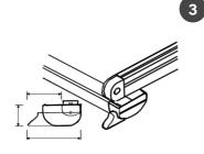
Extruded aluminium profile for rainwater collection, only for sloped versions, fixed to the end support tube. One drainage per runner. Down pipes not provided.
