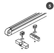
ASHELTA runner complete with sliders, support tube joints, central transmission shaft with bushings.
